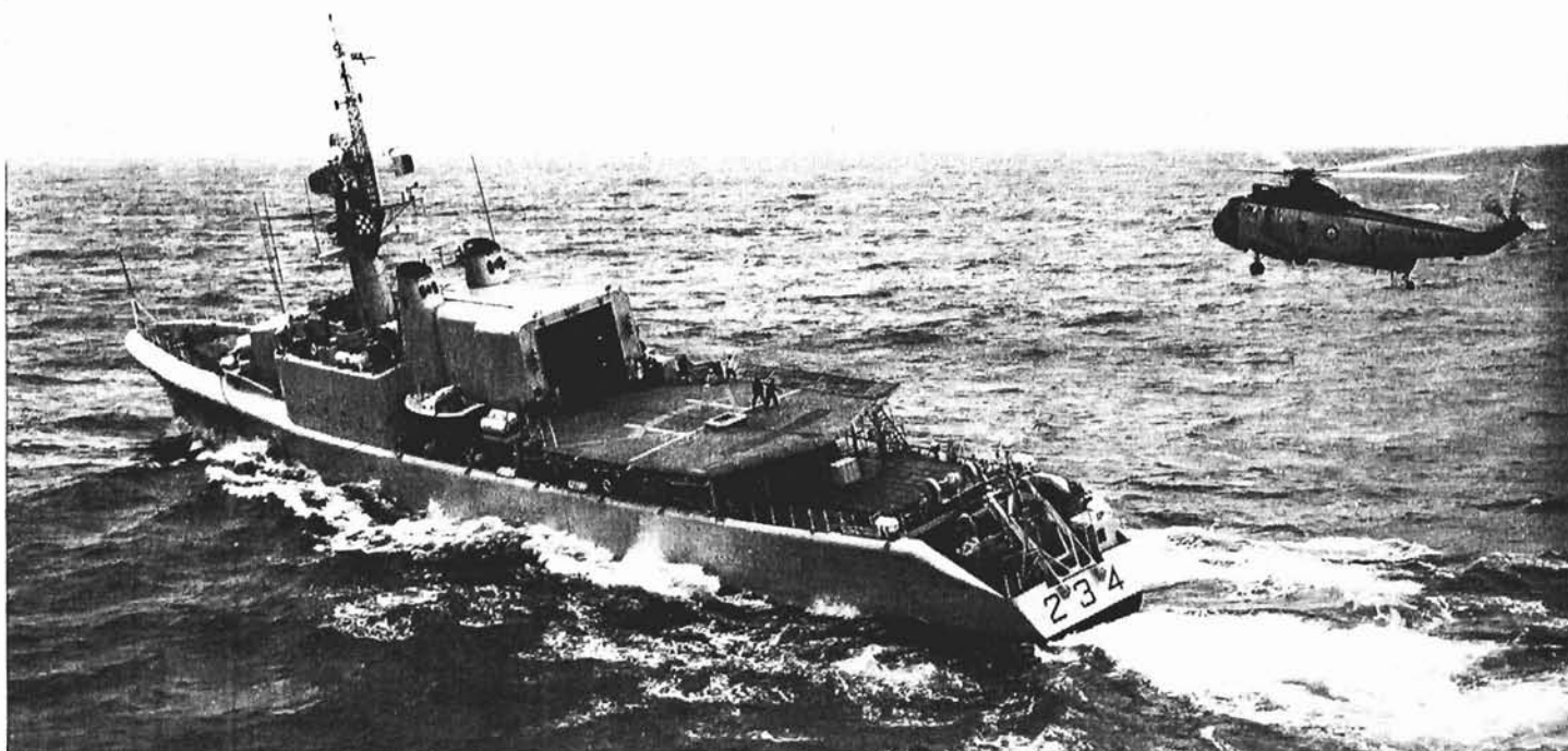
A Sea King helicopter begins its approach to the flight deck of the Assiniboine. Flight deck crewmen wait beside the beartrap device. (DNS-33910)
