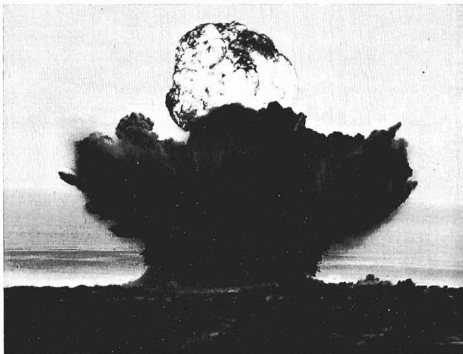
The Second Sailor Hat test charge is detonated on Kahoolawe island, Hawaii, to determine the blast effect on modern ships and weapon system. The 500-ton charge was detonated by the U.S. Navy at 3:21 pm, April 16, one of the ships exposed to the blast being HMCS Fraser . The Sailor Hat tests, conducted by the USN under the sponsorship of the Defence Atomic Support Agency, will end with the third and final detonation in mid-June. The first detonation occurred on Feb. 6, with the Fraser present on that occasion. (U.S. Navy Photo)
