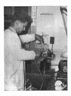
In the laboratory in the dental clinic at HMCS "Naden" Sergeant Technician William Powers, of Winnipeg, operates a casting machine used in making complete or partial dentures. (E-9699)
