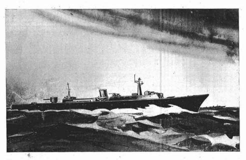
Above is an artist's conception of the RCN anti-submarine escort vessel, working drawings of which are now being prepared. It is expected that keels for three of the new ships will be laid down at the end of the year or early in 1950. The escort vessels will have steel hulls and aluminium superstructures and bridges and will be driven by steam turbines. Accommodation will be provided for a crew of more than 250. ("Crowsnest," July 1949.)
