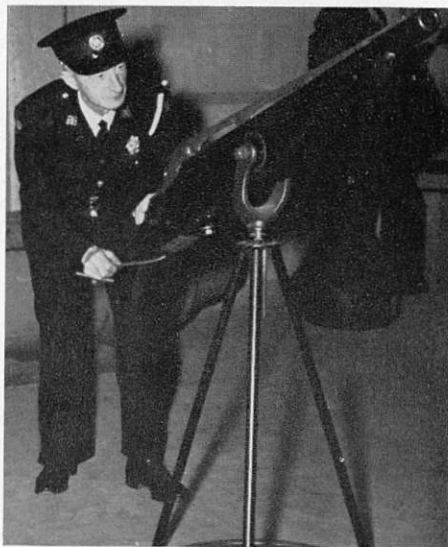
A line throwing gun used for many years on Sable Island for throwing lines to ships trapped in the treacherous sands is now one of the exhibits at the Maritime Museum in H.M.C. Dockyard, Halifax. Commissionaire A. H. Grant, museum guard, demonstrates how the gun is fired.
