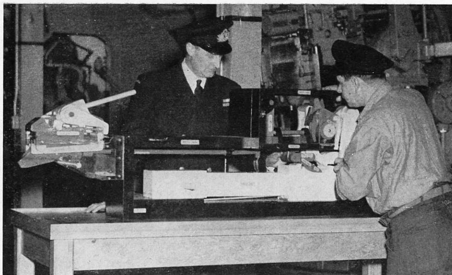
The Navy's new Ordnance School takes advantage of all methods of instruction and training. Checking over a wood and plastic working model of a 20-mm. gun are Ord. Lieut. George Y. Moyes, gunnery maintenance training officer, and CPO Jack Anslow. The model enables instructors to show what happens inside the gun when it is being fired. (E-12717).
