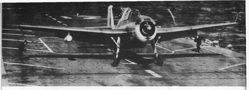
An Avenger aircraft has just landed on the "Magnificent's" flight deck and aircraft handlers rush out to remove the arrester wire from the tail hook.
