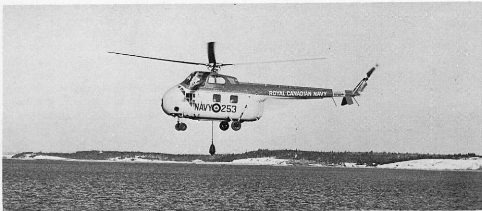
A Sikorsky helicopter of HS 50, the RCN's helicopter anti-submarine unit, hovers over a practice area off the coast of Nova Scotia preparatory to lowering its "pinging" and listening gear into the sea. (DNS-15082)
