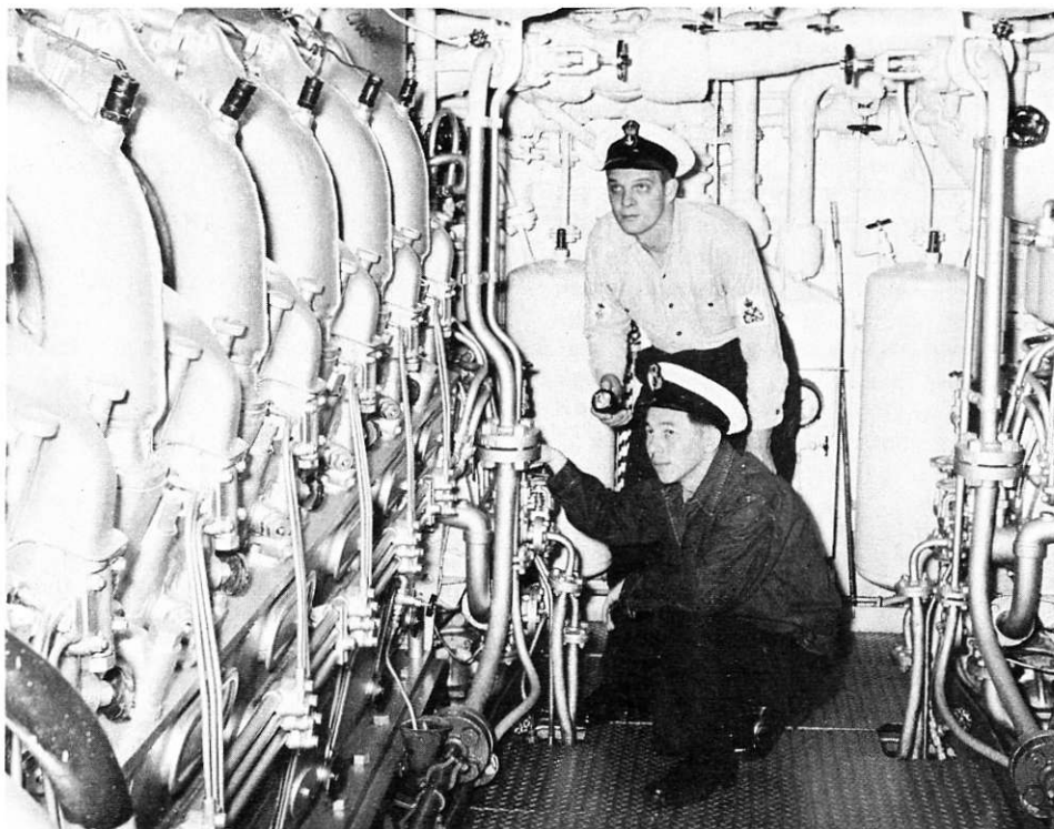
Canada's wood and aluminum minesweepers are propelled by two 1,200 horsepower diesels. Checking one in HMCS Resolute are PO Myron L. Bennett, top, in charge of the watch, and CPO Roy J. Osborne, chief engineering artificer of the ship. The photo was taken while the Resolute was senior ship of NATO minesweeping forces in Sweep Clear V off Shelburne, N.S. (CS-574)
