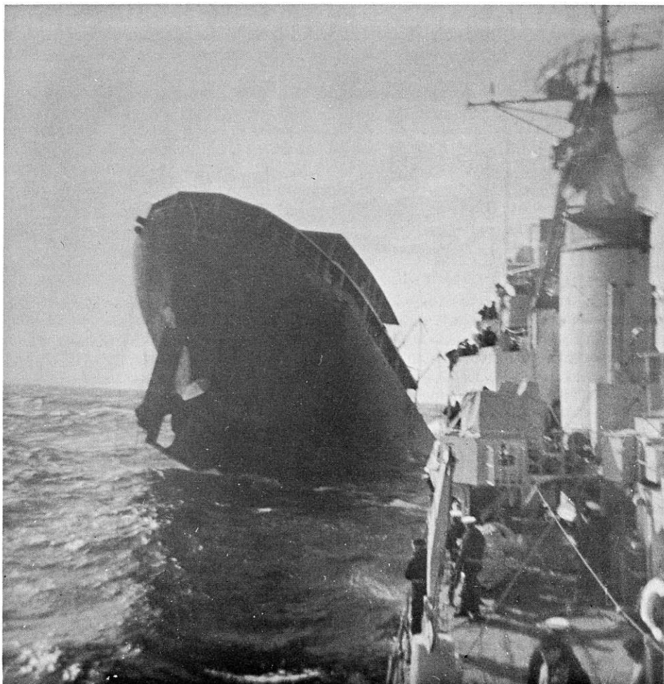
The Athabaskan approaches the stern section of the tank Amphialos, which broke in two in the North Atlantic on March 1, 1964. (HS-74376)
