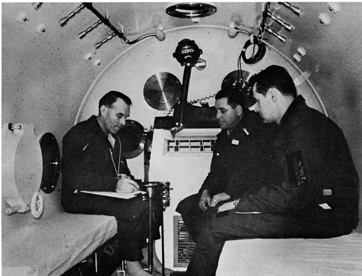
Diving computers are cross-calibrated during simulated dives in the hyperbaric chamber at Toronto General Hospital. Surgeon Lt.-Cdr. D. J. Kidd jots down figures while CPO J. H. Wilson and Ldg. Sea. W. E. Nehring act as guinea pigs. Ldg. Sea. Nehring has contributed greatly to the developmental program and has made variants of the computer to his own design.
