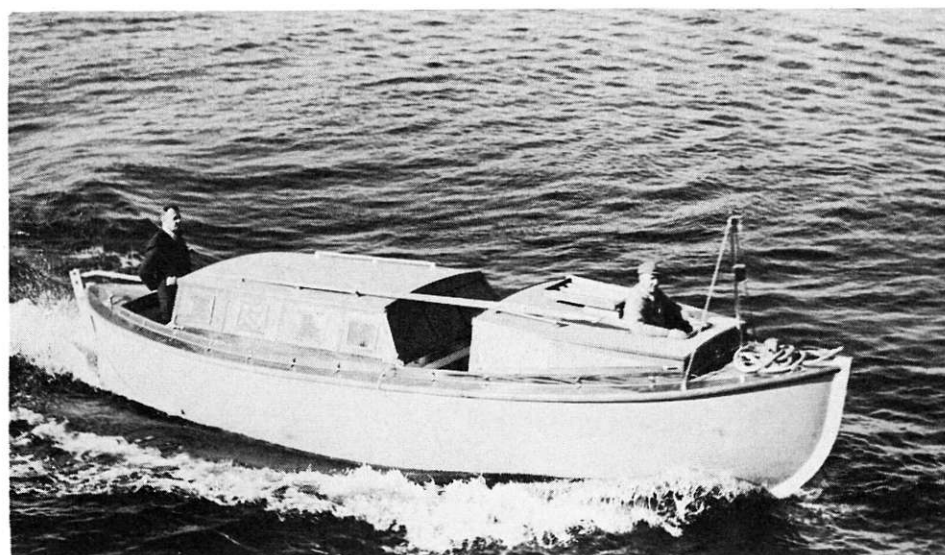
The 27-foot Canadian motor sea boat is shown going through its paces at the Arnprior "regatta". This boat is a modification of the Royal Navy motor seaboat, the main difference being a whaler stern, greater power and omission of the mast and sails. (O-6008)
