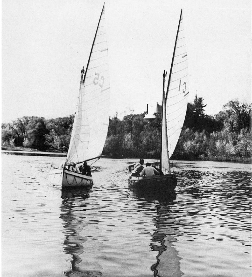
Crews compare the performances of two dinghies under sail. On the left is a prototype 14-foot dinghy built of polyester resin reinforced with fiberglass cloth and mats. It is the first boat of this type of construction to be built for the RCN. (O-6014)
