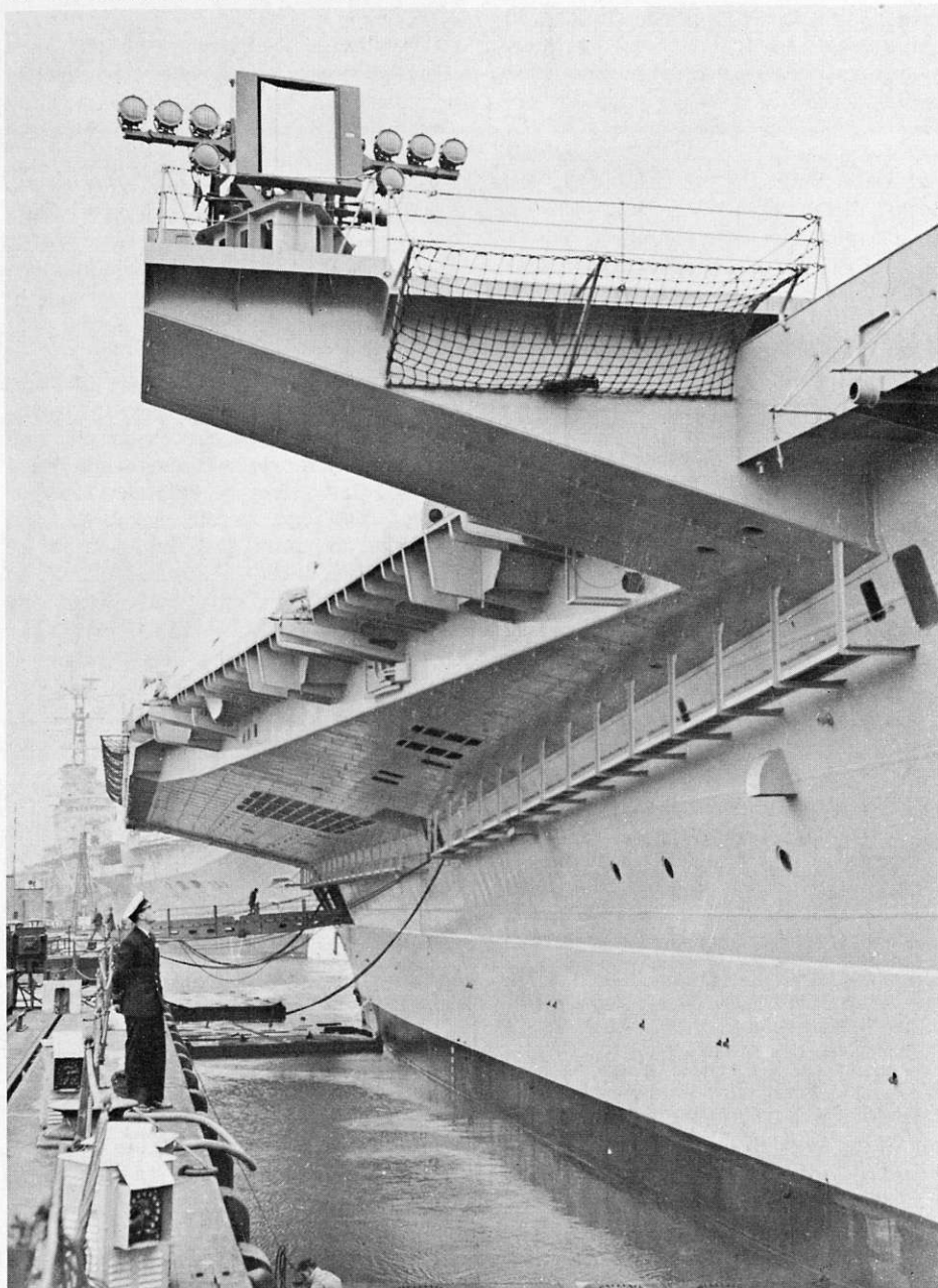
Described by the Royal Navy as the world's most modern aircraft carrier, HMS Victorious is again in service after what turned out to be one of the world's longest refits—seven years. In addition to all the latest flight aids, she has fantastically powerful radar and a filter system to provide fresh air for control rooms in the event of atomic attack. Her angled deck overhangs the ship's side by more than 35 feet and the landing mirrors have had to be installed on their own little deck, as shown. (Photo courtesy U.K. Information Office.) See story on page ten.
