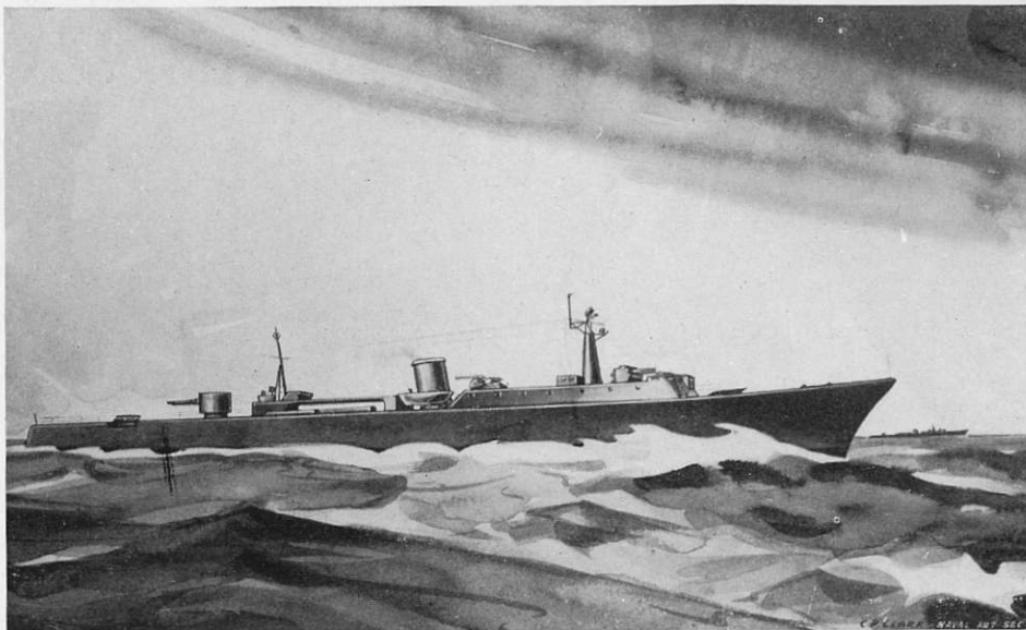
Above is an artist's conception of the RCN anti-submarine escort vessel, working drawings of which are now being prepared. It is expected that keels for three of the new ships will be laid down at the end of the year or early in 1950. The escort vessels will have steel hulls and aluminium superstructures and bridges and will be driven by steam turbines. Accommodation will be provided for a crew of more than 250. ("Crownsnest," July 1949.)
